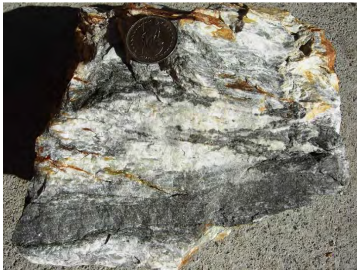
Figure 7.6 High-Grade Pyrite-Arsenopyrite Bands within Strongly Silicified Sericitic Schist
