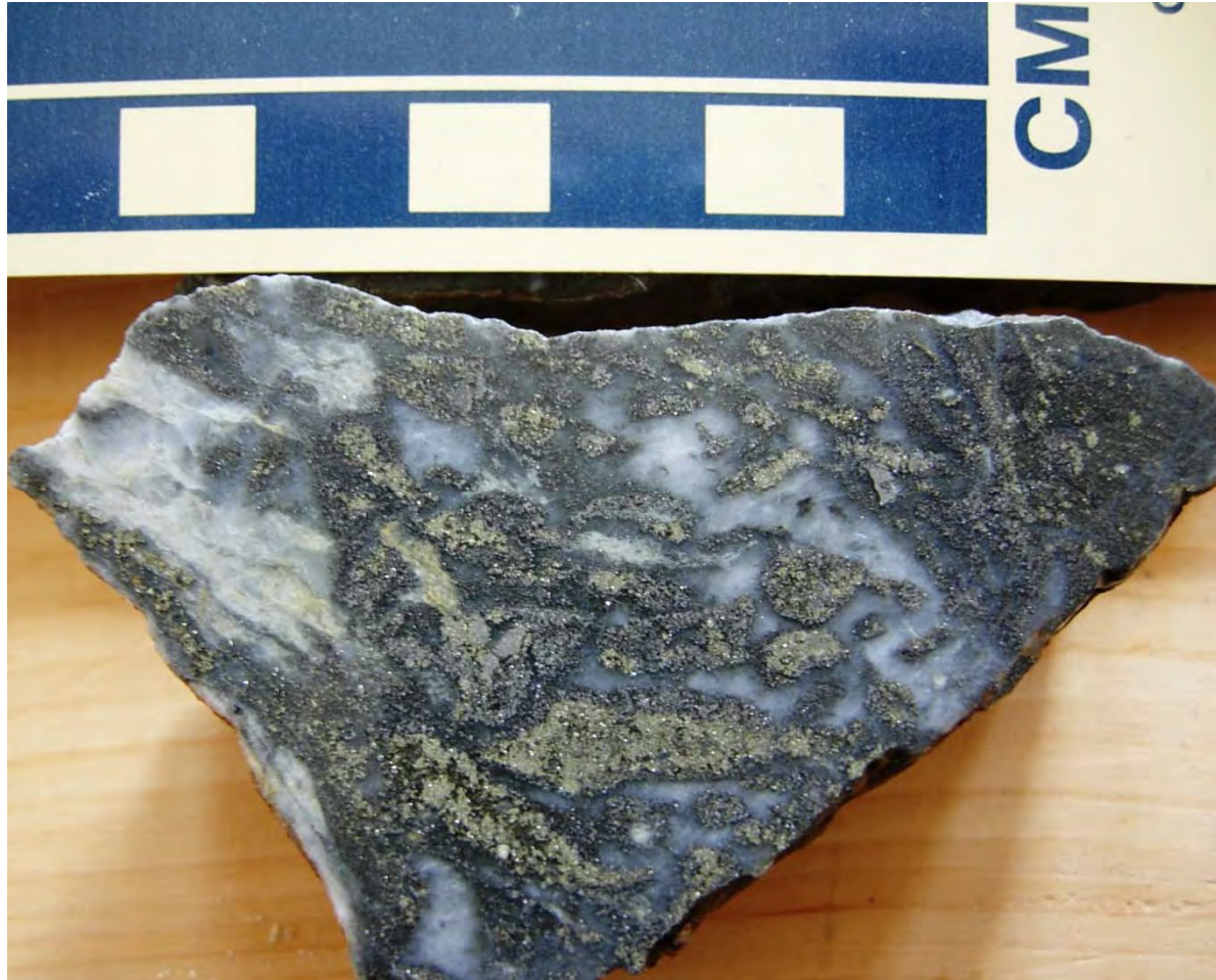
Figure 7.7 Sulfide-Rich Quartz-Sericite Schist
